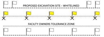
Observe the facility owner's Tolerance Zone and leave at least 1 metre of tolerance on either side of the located underground facility. Excavation within the Tolerance Zone requires care for protection of the underground facilities. Based on climate or geographic conditions, they include:
